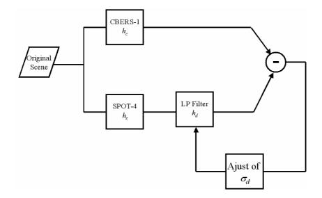
Fig.11 block diagram of low-resolution image simulation
