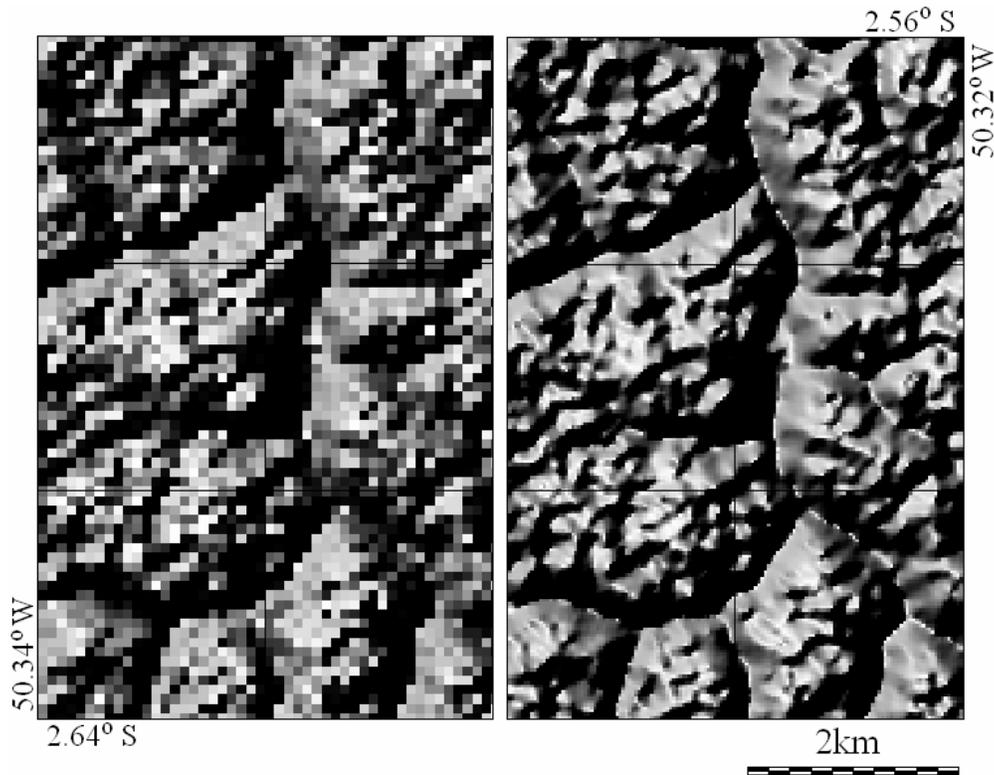
Figure 1: Shaded relief of SRTM-90m original data (left) and resampled DEM (right).
