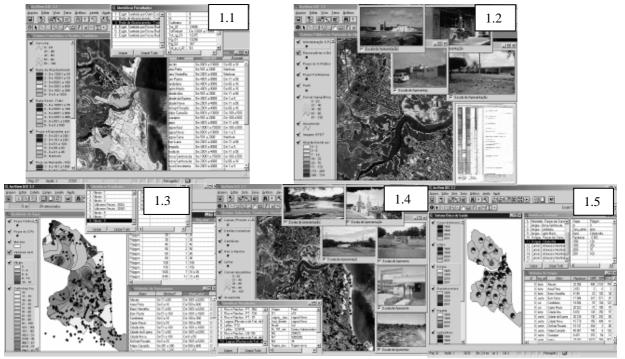
**Fig. 01** - The Water Management System GIS is composed for five main themes: which include IBGE data (1.1); System of Public and Private Provisioning (1.2); Water Quality (1.3); Cemeteries, Industrial Districts, Ponds, Flooded and Garbage (1.4); Data from Municipal General Office of Health (1.5).
