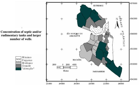
**Fig. 6** - Areas of larger concentration in septic tanks and/or rudimentary and larger number of wells. These were identified in agreement with the base of data of the census section that has answered to this criterion. The hachure of dark gray tone shows the neighborhoods under risk in relation to the quality of the water.
