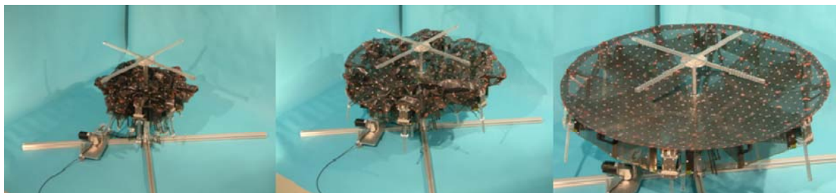
Figure 5. Bread-board antenna deployment procedure
