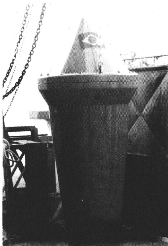
Fig. 1 - View of buoy shortly after its construction. The antenna is located inside the top cone, the transmitter is just inside the widest part of the hull, and the power supply is in the bottom of the buoy.
