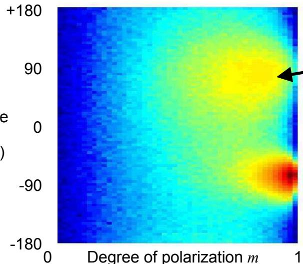
Expected opposite-sense phase signal in response to circularly polarized transmissions, indicating single-bounce (specular) or triple-bounce backscatter
