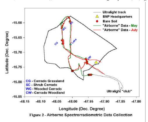
**Data Processing & Analysis Approach** – The atmospheric free, nadir looking spectroradiometric data, processed to surface reflectance values traceable to a NIST<sup>1</sup> reflectance standard, was convoluted to the MODIS bandpasses and converted to the Normalized Difference Vegetation Index (NDVI) and the Enhanced Vegetation Index (EVI), according to the following equations:
